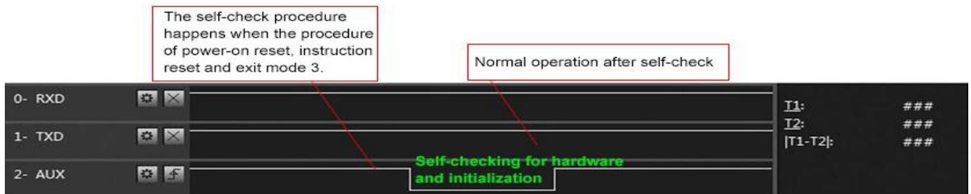
Timing Sequence Diagram of AUX when self-check
